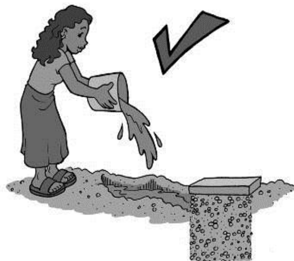
Wastewater going into soak pit
