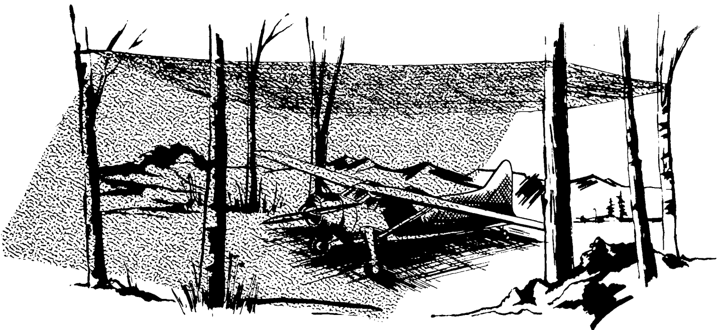
(2) If additional camouflage is needed, to protect from oblique observation, a garnished twine net can be hung from the exposed sides.
