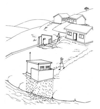
The chamber (if it is a compost toilet) should be at least 2½ metres above the groundwater. Keep in mind that water levels are much higher in the wet season than in the dry season. When there is a risk of groundwater pollution from pit toilets, build an above-ground toilet. Any toilet should be at least 20 metres from rivers, lakes, springs, streams and wells.
