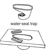
water-seal trap set in concrete platform
