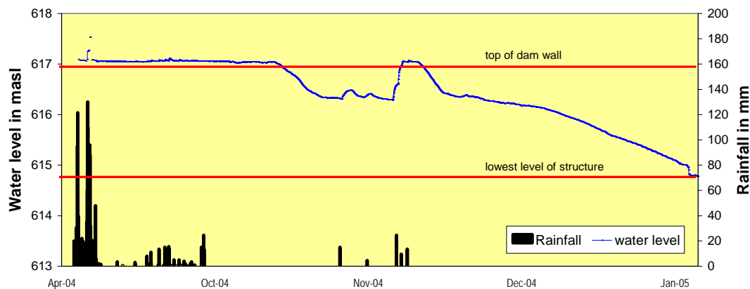
Figure2 Response of the water level at Chikhalgaon (CD3) to rainfall in the 2004.
