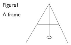
When the two feet of the A are at the same height, the string should hang exactly in the middle. Measure and mark this position in the middle of the horizontal pole of the A frame.
