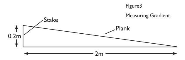
For example, the slope above would be  $0.2 / 2 \times 100\% = 10\%$  gradient
