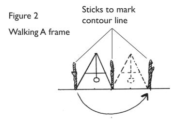
Point A of the A frame is swung to Point B keeping C in a fixed position.
