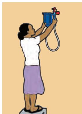
9. Place cartridge back in holder.
