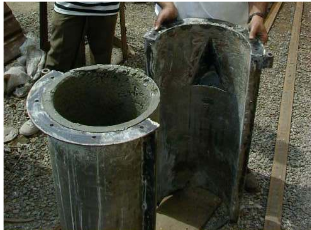
Carefully, pull the two halves apart. The shell with the nose can be more easily removed by tilting the filter backwards while first pulling the shell outwards from the base.
