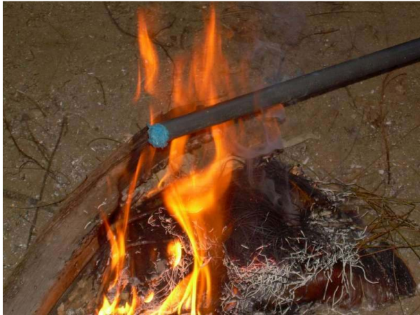
Heat the pipe over a fire, turning continuously. When it becomes floppy, bend it to the desired shape and fix the shape by dousing with water.
