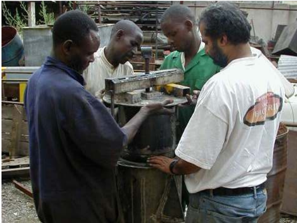
At a certain stage, you can remove the inner core by hand.
