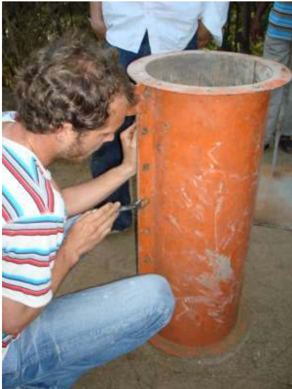
Assemble the two outer halves of the mould using the bolts.
