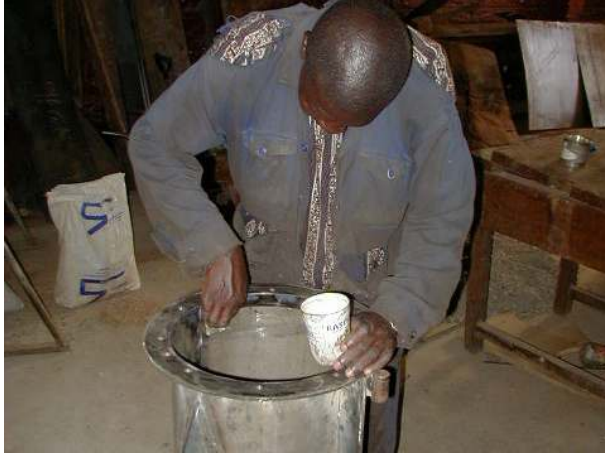
Also grease the inner sides of the outer shell.
