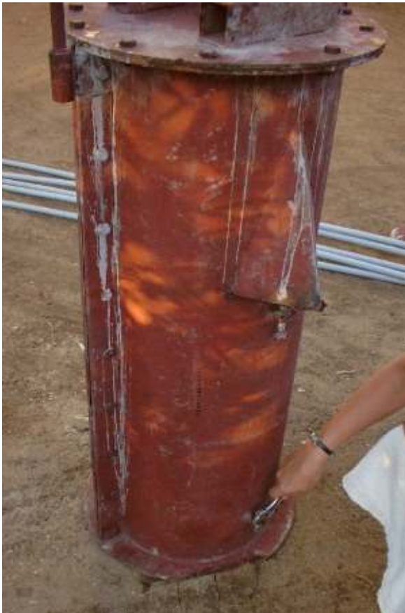
Remove the nose plate, and unscrew the bolt near the base that secured the PVC pipe.
