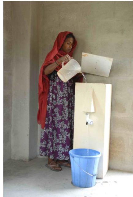
Figure 1: Domestic bio-sand filter used in Bangladesh. Photo: Practical Action Bangladesh.
