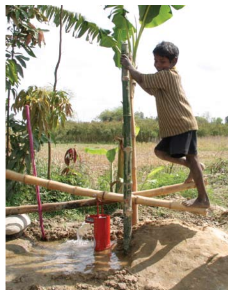
Treadle pump India showing bamboo treadles and metal cylinders. On each stroke, the piston in one of the cylinders drives water into an irrigation canal
