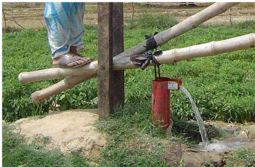
Figure 4: An example of a class I lever in the Bangladesh treadle pump [20]
