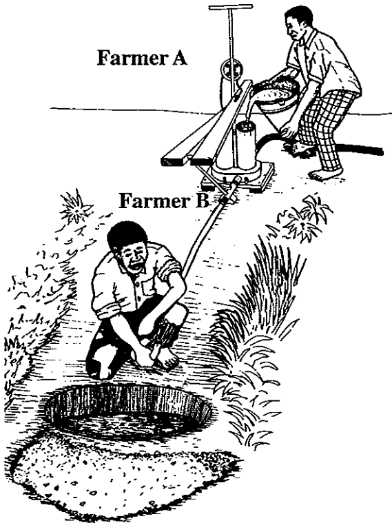
Figure 11: Filling the cylinder while holding the end of the suction hose up
