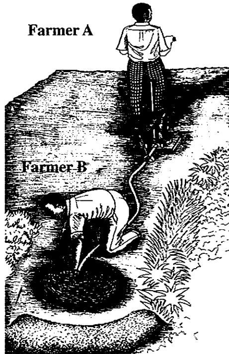
Figure 12: Treadling rapidly after placing the end of the suction hose under water
