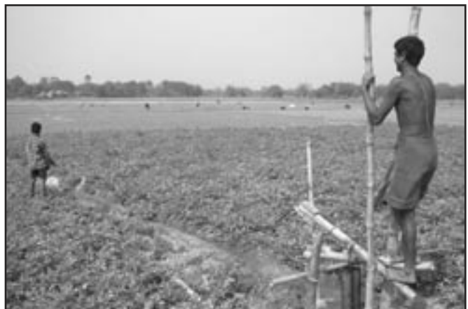
Photo-6: Man irrigating potato farm by using treadle pump in Chilkir hat, Kothwali block
