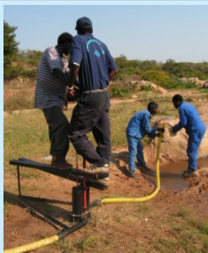
FAO small-scale irrigation projects promote appropriate technology such as drip kits and treadle pumps (the latter is shown above).
