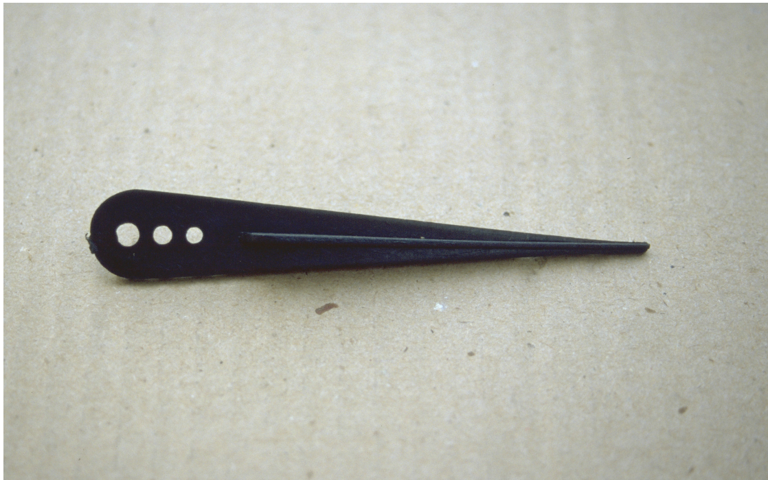
Figure 16: The plastic sticks are made of LLDPE (linear low density polyethylene) and are not strong enough to resist dry and hard soil conditions.
