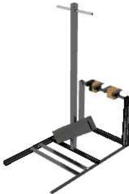
Figure 4.4: Frame with rocker-arm and treadle pivot system
