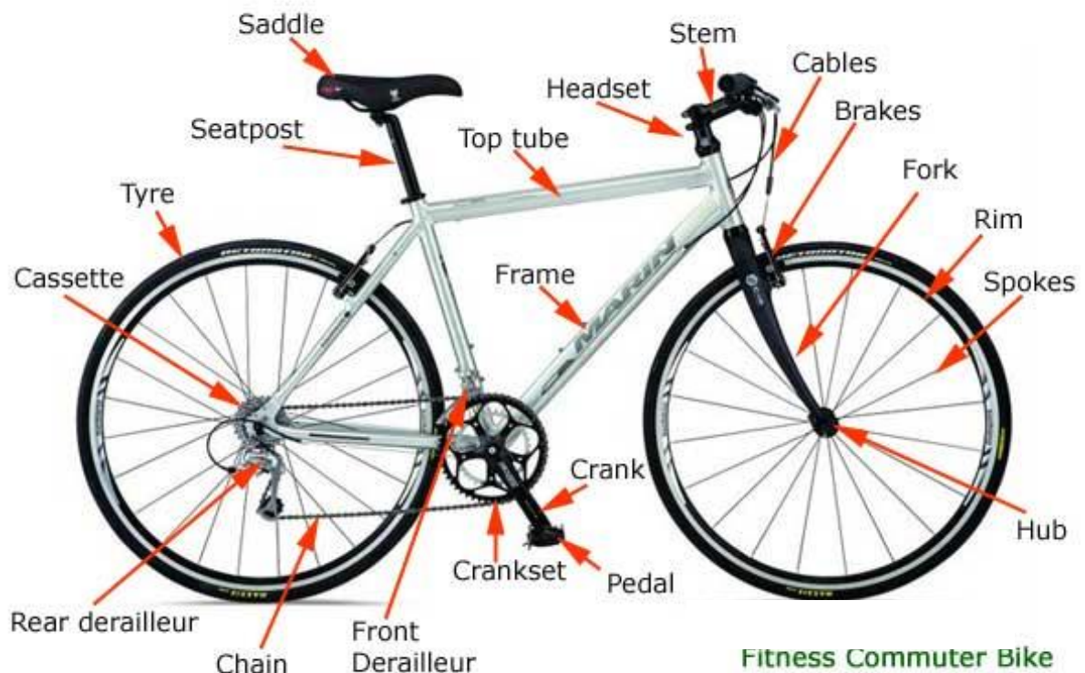
Figure 35. Basic, and non-basic, bike components
