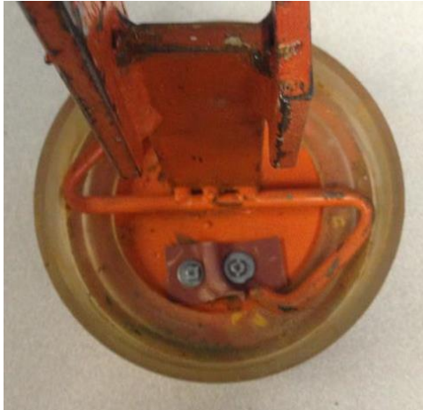
Figure 58. Piston Seal Rod to Seal Interaction
