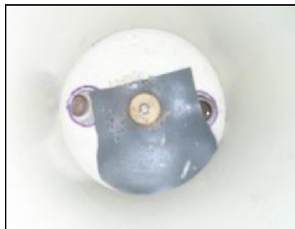
Figure 18. Flapper valve made of thin rubber
