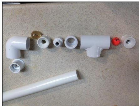
Figure 20. Exploded view of a homemade ball check valve
