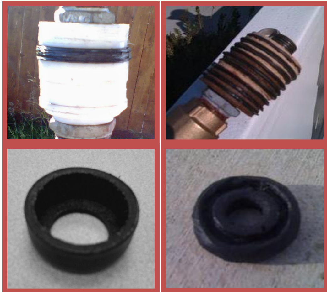
Figure 14. Seal Types. Top Row: flat “O” seal and labyrinth seal Bottom Row: cup seal and “U” Seal
