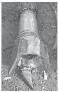
Teeths of drill bit from steel from truck springs
