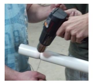
2) Locate the large 4" diameter PVC pipe section (#3 in picture). Using a saw or drill, cut a 2" a circular hole leaving about 1" of clearance from the bottom of the large PVC pipe. Cut an identical hole across from the new hole on the opposite side. Now insert the grooved 2" diameter PVC pipe though the cut holes in the large PVC pipe. Using PVC primer and
