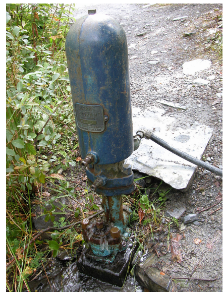
Figure 1: A hydraulic ram that drives a fountain at the Centre for Alternative Technology
