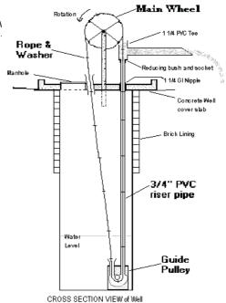
Figure 7: Rope and washer pump.
