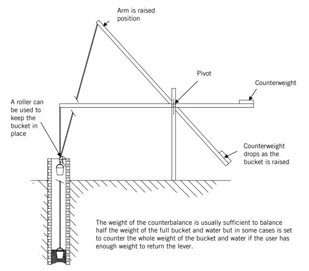
Figure 1: A counterpoise lifting device, also known as a shadouf, over an open well. A counterbalance helps lift the bucket of water.
