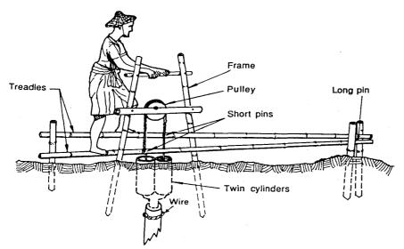
Figure 5: Treadle pump
