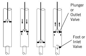
Figure 2: How most types of pump cylinders work.
