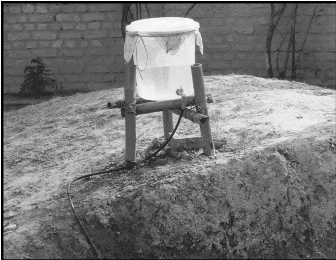
The bucket kit for low cost drip irrigation in the test laboratory of IDE India near New Delhi. A simple product with a long trial and error phase to make it suited to the needs of poor horticulturists.
