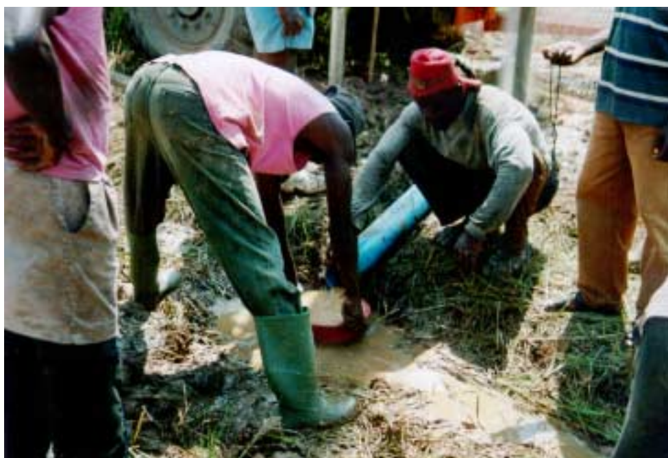
Figure 6.1 Measuring yield during airlift.
