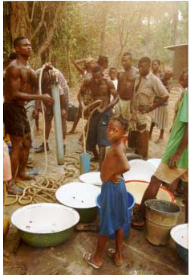
Figure 6.2 Community members helping with a bailer test in Edumoga, Nigeria,
