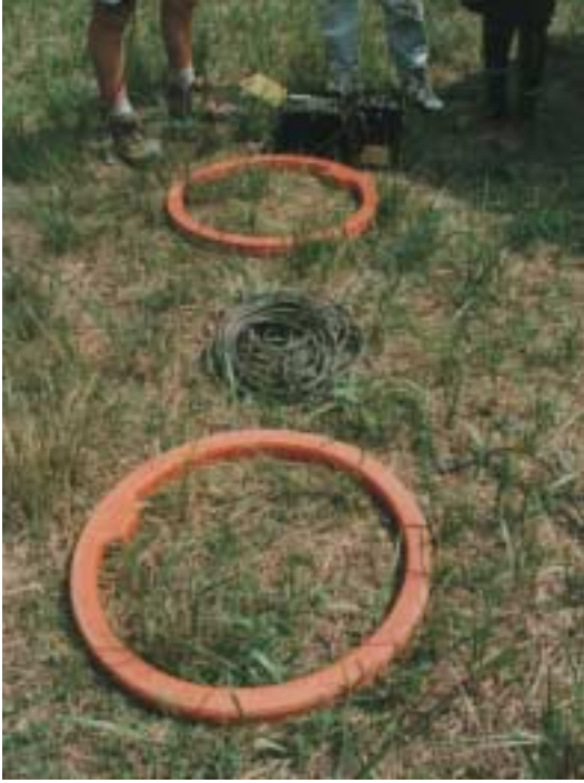
Figure 4.8 The EM34 equipment, comprising two coils, a connecting cable, transmitter and receiver.
