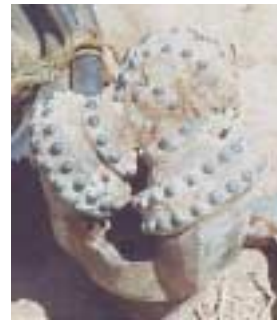
Tricone rock roller bit with tungsten carbide teeth
