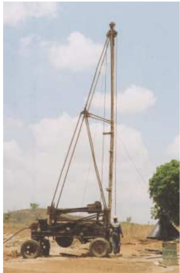
Photograph of percussion rig in use.
