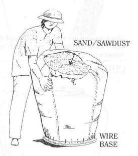
When the base is dry, place the form on top of the base. Then fill the form with sand/ sawdust. Mould the form until you are happy with the shape. You are ready to plaster.
