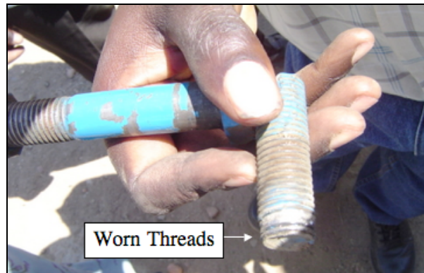
Figure 82. Hitch incorrectly inserted in top Figure 83. Roll-axis bolt has worn threads
