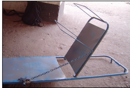
Figure 38. Chain secured when reclined
