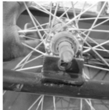
Figure 17: Push the axle as far into the slots as possible and tighten the nuts so the wheel does not fall off.
