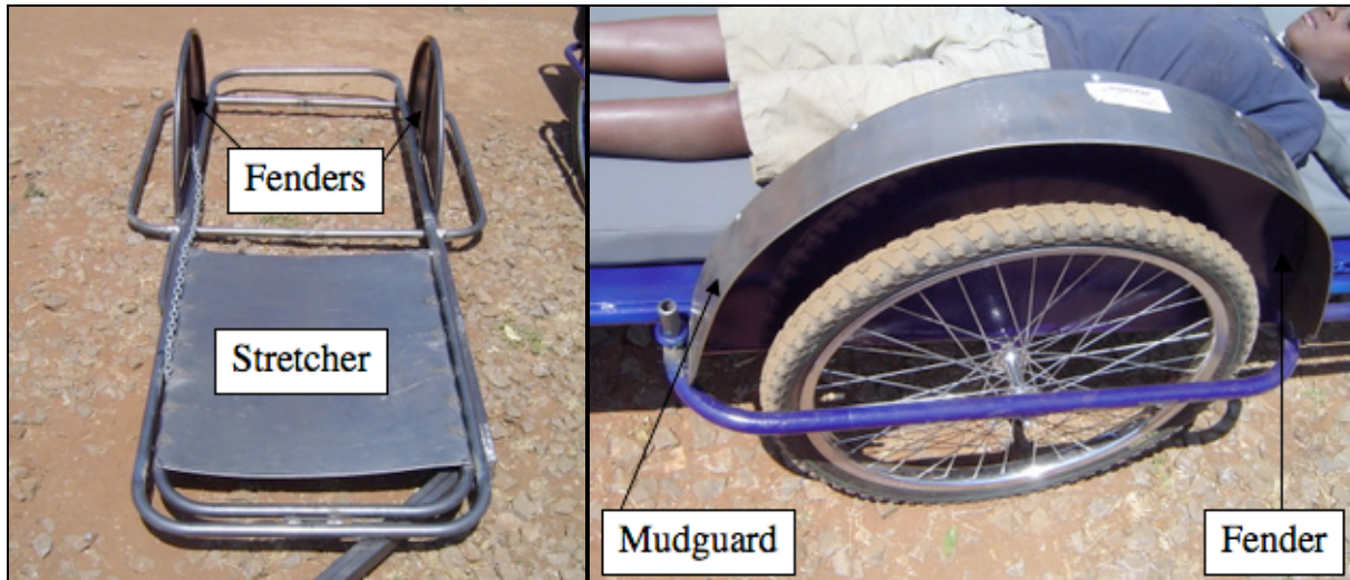
Figure 60. a) Fenders confine the stretcher, and b) fender and mudguard protect patient
