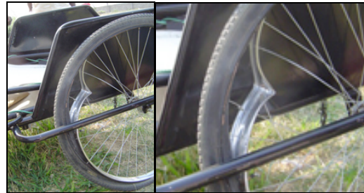
Figure 54. Trailer wheel rim collapse
