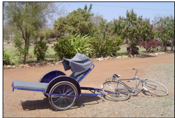
Figure 78. Angle change causes interference Figure 79. Correct design allows bike to fall
