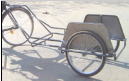
Figure 53. Beta tow bar reinforced
