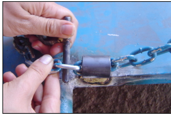
Figure 36. Lock new link to change angle
