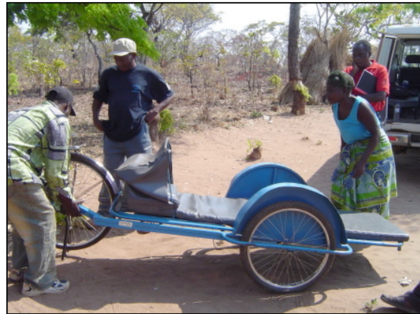
Figure 87. Trailer rear is tilted downwards
