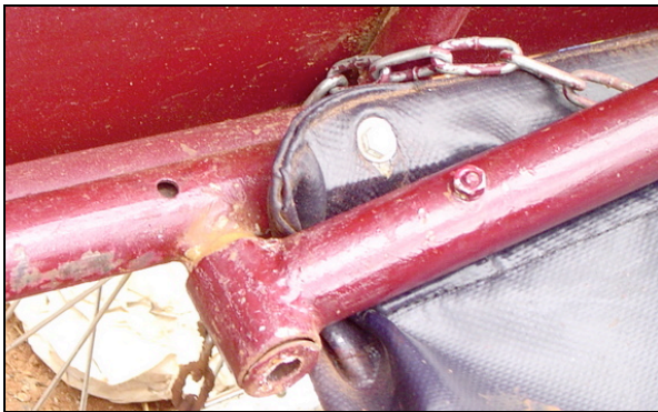
Figure 27. Bolts and nuts hold tarp to frame
