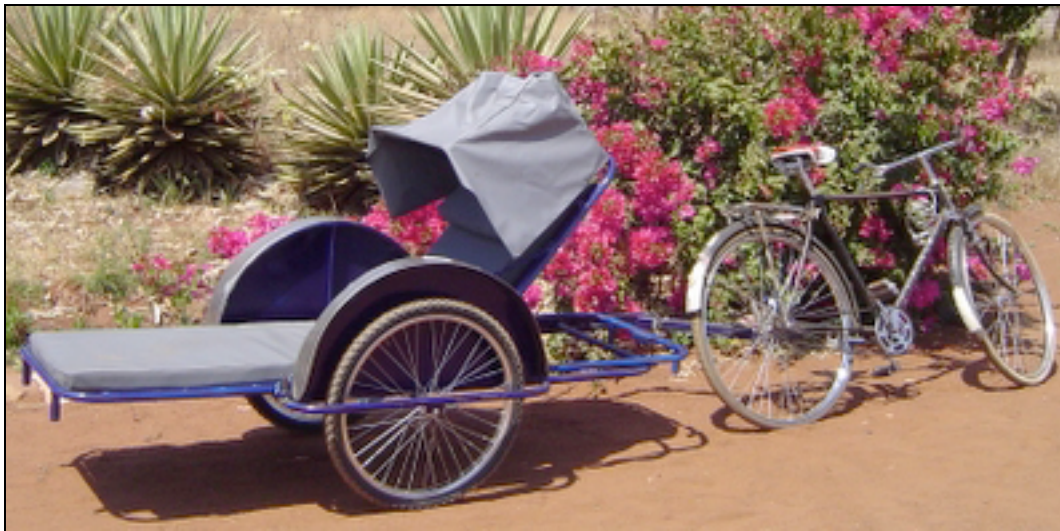
Figure 4. Gamma Zambulance attached to a bicycle.
