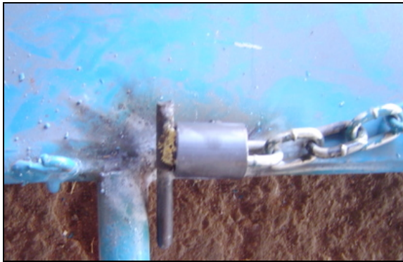
Figure 35. Chain end is secured by a rod
