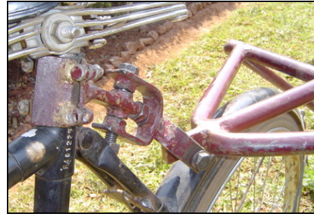
Figure 50. Deformed Beta hitch
