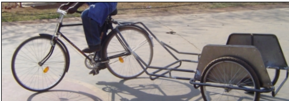
Figure 48. Beta tow bar and bicycle rear wheel interference
