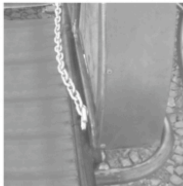
Figure 13: Hook the chain even when it is not in use to prevent it from dragging or hitting the wheel
