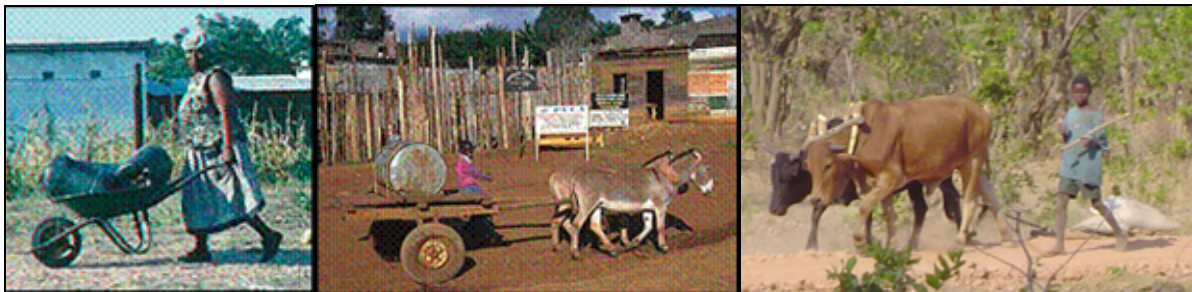
Figure 1. Wheelbarrows, animal-drawn carts, and ox sledges are common IMTs.
