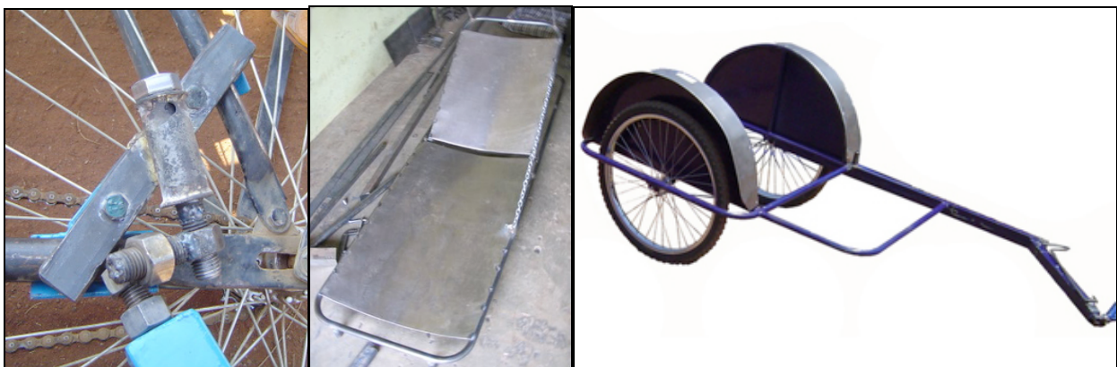
Figure 19. a) Gamma nut and bolt hitch, b) sheet metal stretcher bed, and c) planar trailer
