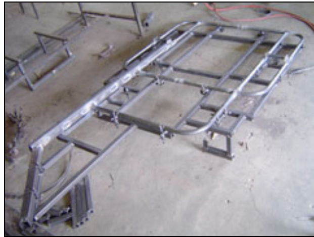
Figure 10. Welded trailer on fixture
