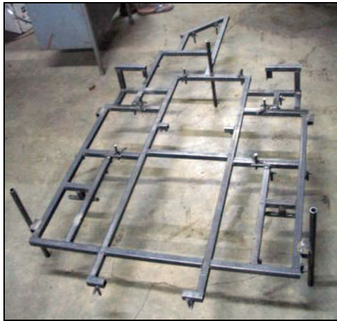
Figure 9. Welding fixture alone
