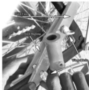
Figure 7: Tighten the clamp face to the clamp backing with the winged-bolts. CLAMP should NOT MOVE. DO NOT OVERTIGHTEN or bicycle frame will be dented.
