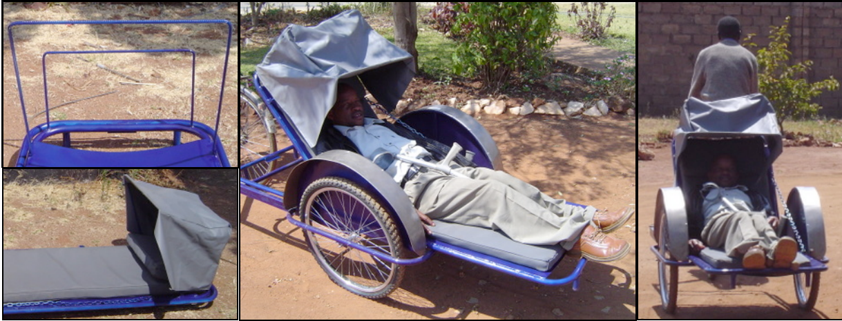
Figure 42. a) Canopy frame, b) and c) Canopy protects from sun, but not rain or stigma
