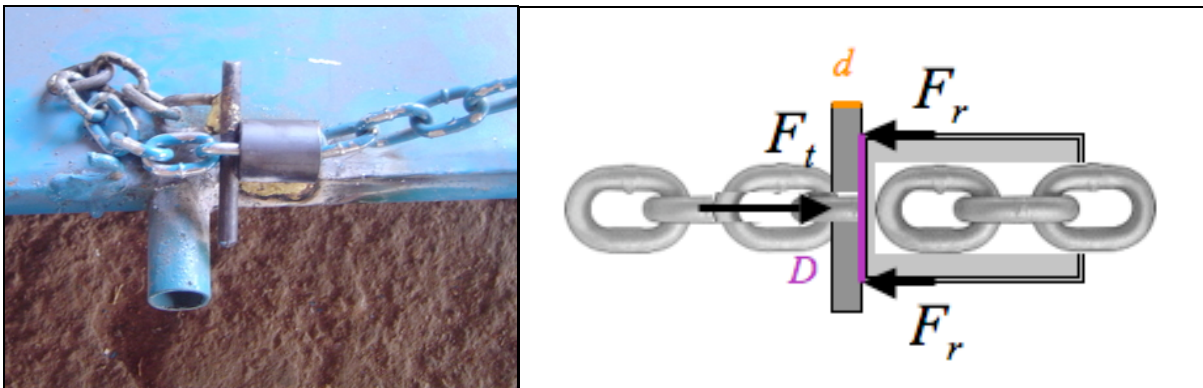
Figure 104. Chain lock schematic of a simply supported beam with a central point load
