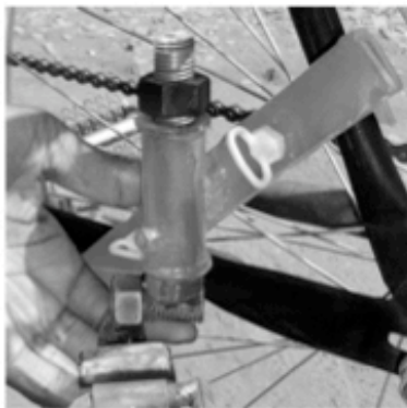
Figure 8: Put the LARGE (M16) BOLT into the BOTTOM of the TUBE and screw on the nut until there is only a SMALL GAP. The BOLT should TURN freely.
