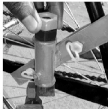
Figure 9: Hold the 1 st nut, & tighten the top nut against the 2 nd nut so the TWO NUTS DO NOT MOVE.
