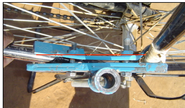
Figure 75. Over-tightening bends clamp
