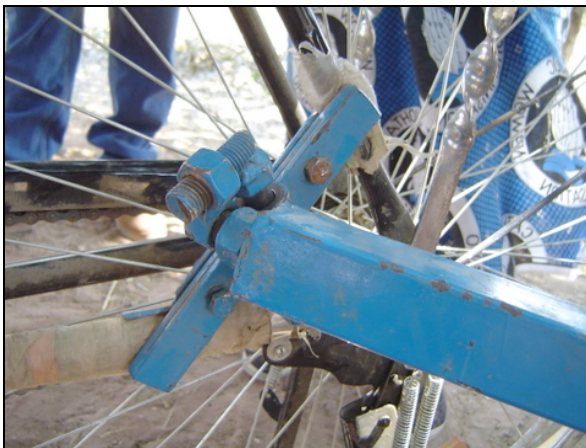
Figure 86. Hitch incorrectly inserted in top
