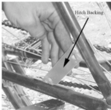
Figure 6: The clamp backing should be on the INSIDE of the frame on the LEFT side of the bike, (LONG ARM is on the BOTTOM, & SHORT ARM is on the TOP).
