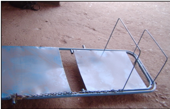
Figure 37. Chain secured when lying down
