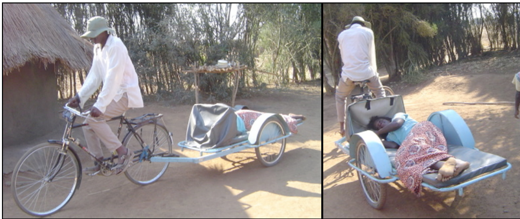
Figure 29. The Gamma ambulance transports a patient from her home to a clinic
