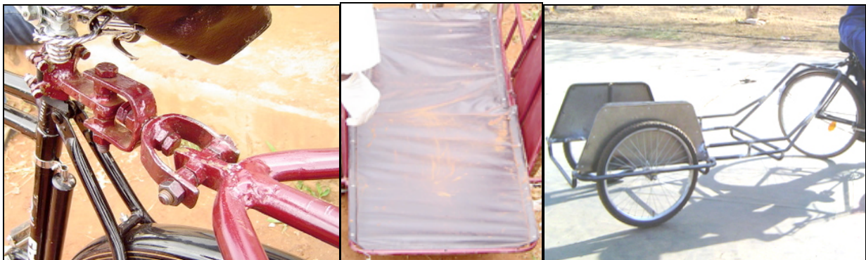
Figure 18. a) Beta U-joint hitch, b) PVC tarpaulin stretcher bed, and c) reinforced trailer
