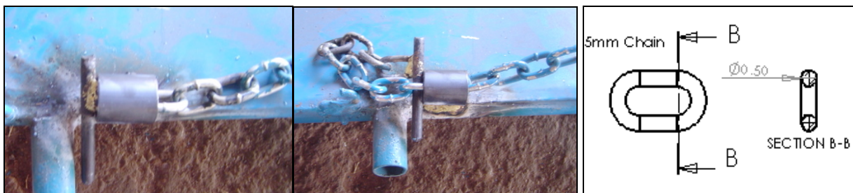
Figure 101. a) Chain secured when backrest is flat or inclined, b) Chain gauge schematic
