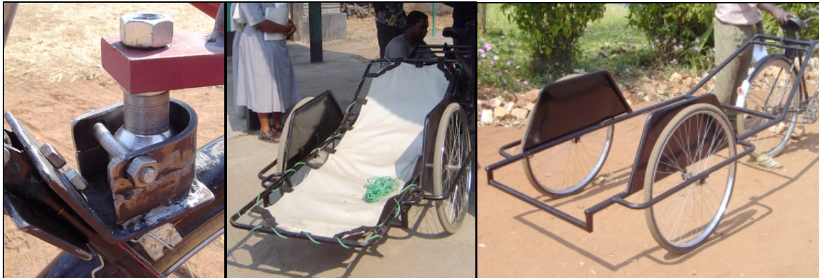
Figure 17. a) Alpha ball joint hitch, b) canvas stretcher bed, and c) 32mm OD tube trailer
