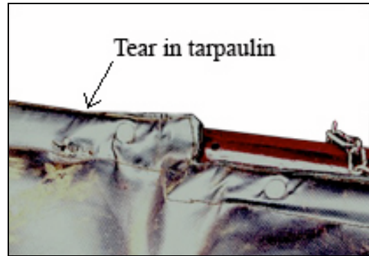
Figure 28. Metal in hem causes tears
