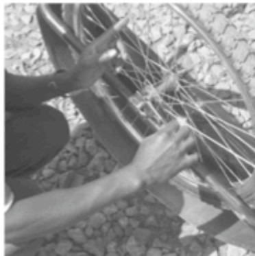
Figure 16: Use front hubs with 36 spoke holes. Make sure the wheels are straight before tightening.
