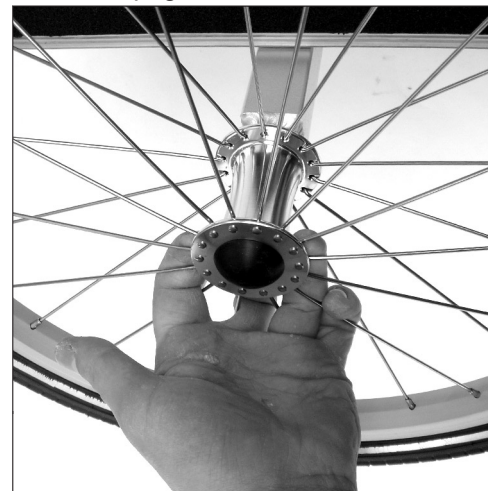
10. Pull at the wheel to ensure it is secure. See page 8 if it isn't
