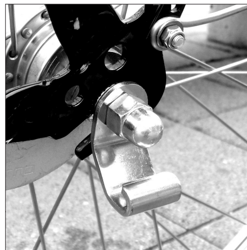
12. With nutted axles the bracket sits between essential washers and the nut
