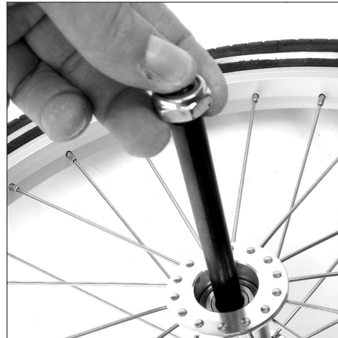
6. Push the button on the end of the axle, and insert into the wheel.
