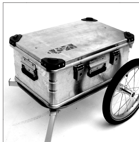
18. Box bolted to the load bed
