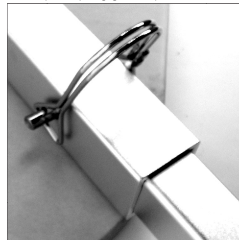
5. Slide the shaft pin through the frame and clip its spring gate in place
