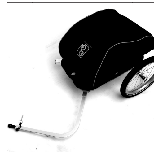
17. Bag. Ortlieb Rack Pack compression straps feed through the Load bed holes to easily hold the bag on the trailer
