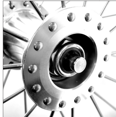
7. The nutted end of the axle should sit in the recessed side of the wheel
