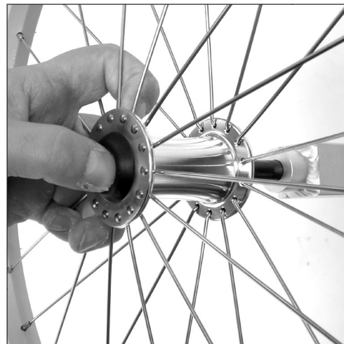
9. Push the center of the hub cap and insert the wheel into the trailer frame
