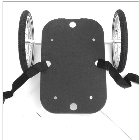
22. Fit straps to the holes. NOTE: Attach one strap with velcro, & one with buckle
