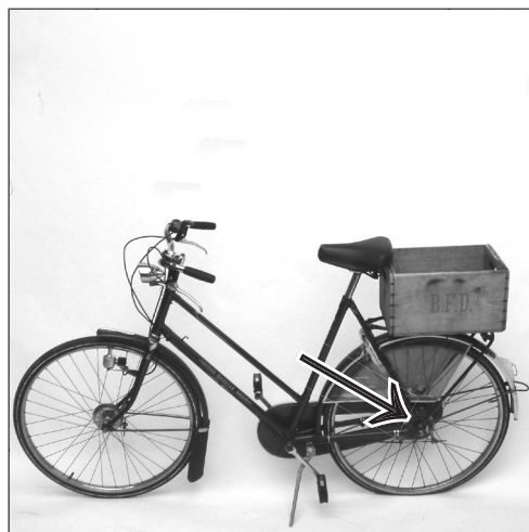
11. The Bike bracket attached to the left chain stay using the rear wheels axle.
