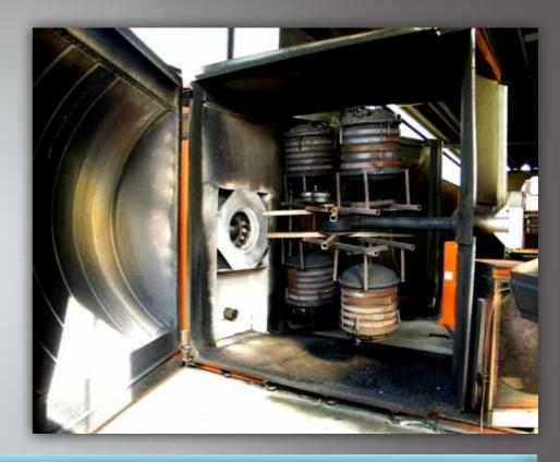
The Hippo roller mould is filled with LLDPE powder & then moved into the oven while rotating in all directions.
