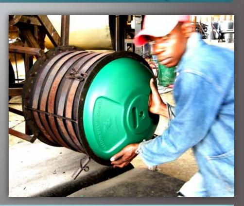
After being heated in the oven the moulds are then cooled while still rotating, after which the completed drum is removed.
