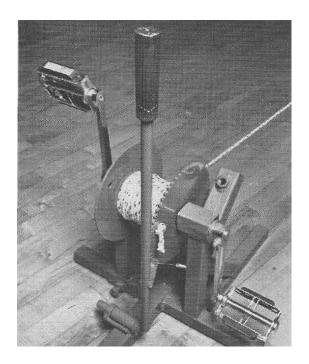
Figure 15: Pedal-powered winch as pictured in Pedal Power (McCullagh 1977)
