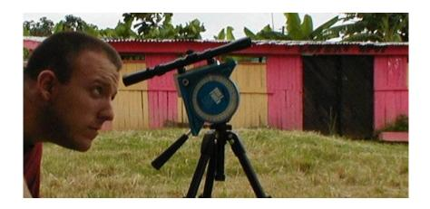
Figure 5: Inclinometer used to verify GPS grade measurements.
