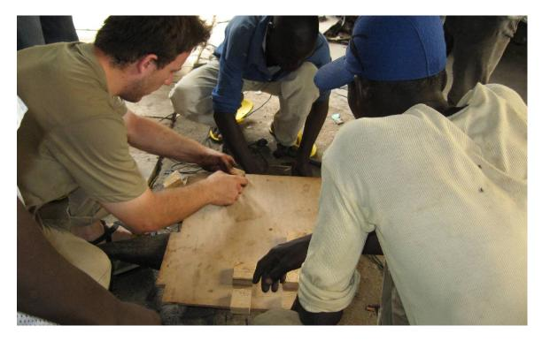
Figure 33: Jigging being constructed from a cheap plank and small scraps of wood.
