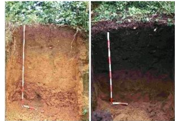
Left a nutrient-poor oxisol; right an oxisol transformed into fertile terra preta - photo courtesy of Bruno Glaser
