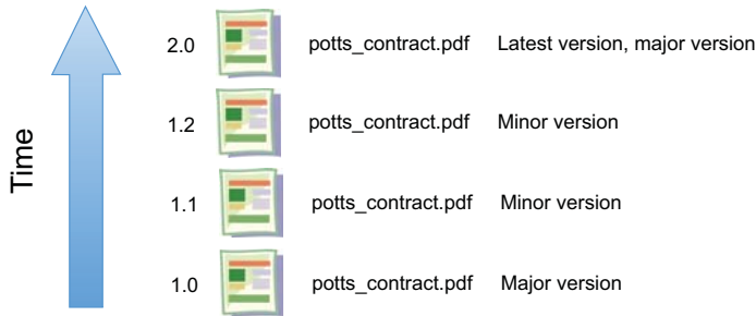
Figure 3.9 Major versions are whole numbers; minor versions are fractions. The latest version is the most recent version in the history.
