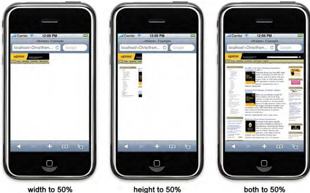
Figure 11–5. If both dimensions are set, the frame is expanded to fit its contents
