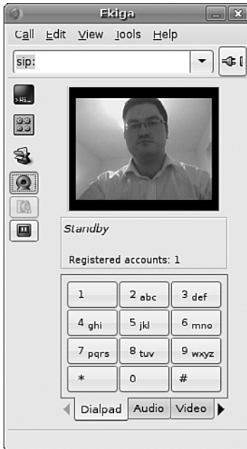
FIGURE 5.19 Ekiga is surprisingly simple to use. A video source is not necessary; a static picture can be used as well.
