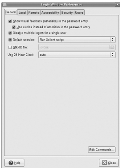
FIGURE 3.7 You use gdmsetup to configure the gdmlogin screen when using gdm as a display manager.
