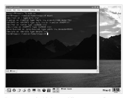
**Figure 14-12.** *Knoppix doesn't load your server's file systems automatically.*
