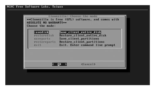
**Figure 2-7.** Select savedisk to write the contents of the entire hard drive to an image file.
