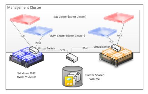
• A typical configuration: iSCSI connectivity to the storage
