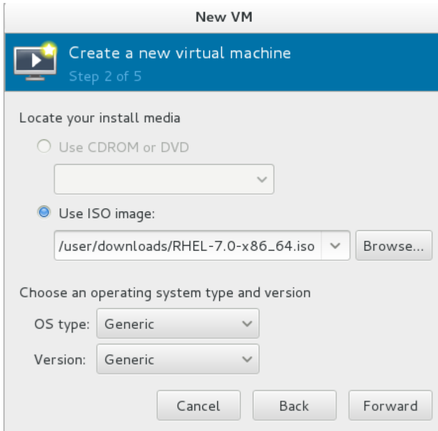
Figure 5.4. Local ISO image installation
