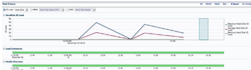
Figure 14-5. Hard disk I/O load on storage cells
