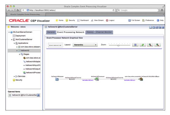
This graphical view is not only a useful visualization aid for understanding the EPN, but also allows you to easily select any of the stages of the EPN.
