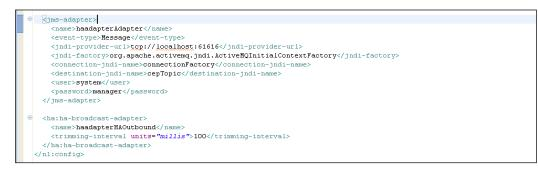
These configurations are persistent and can be changed from the Visualizer tooling or using a JMX client. The JMS adapter's event-type element specifies the event type to which the JMS adapter will convert the JMS messages. The jndi-providerurl is as configured in the ActiveMQ's activemq.xml. The HA adapter's element trimming-interval specifies that the primary server will send trimming message to secondary servers every 100 milliseconds.
