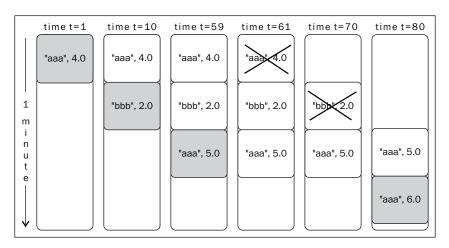
The RANGE operator is a time-based window operator, as it is driven by time. There are several other types of window operators, such as tuple-based and partitioned.
