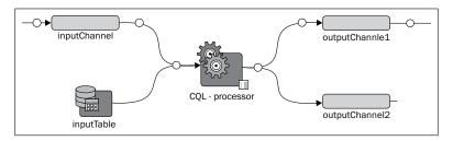
In this case, the channel inputChannel and the table inputTable are the potential sources for query Q1, where as the channel outputChannel1 and outputChannel2 are the potential destinations.
