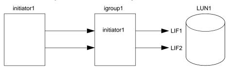
You can limit access to a LUN by binding igroups to port sets. In the following example, initiator1 can access LUN1 through LIF1. However, initiator1 cannot access LUN1 through LIF2 because LIF2 is not in portset1.
