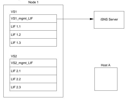
In the next example after the iSNS server completes the registration with the target, Host A can discover all the LIFs for VS1 through the iSNS server as indicated in step 1. After Host A completes the discovery of the LIFs for VS1, Host A can establish a connection with any of the LIFs in VS1 as shown in step 2. Host A is not aware of any of the LIFs in VS2 until the management LIF VS2 mgmt LIF for VS2 registers with the iSNS server.
