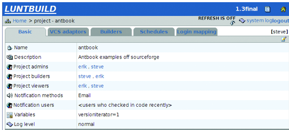
Figure 15.4 A Luntbuild project is bound to a source code repository and can have different builders to build parts of the project on defined schedules.
