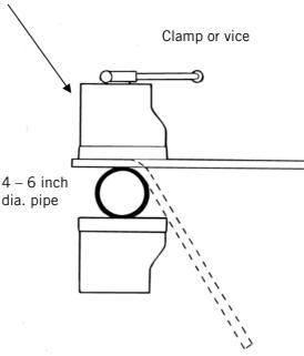
Figure 1: Pipe bending using a clamp or vice
