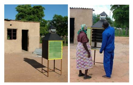
Figure 26. Modified drying tower, the chamber heats up drawing air in at the back and out through the turret at the top.
