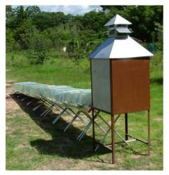
Figure 25. Drying tower with heating funnel 2) Modified tower (Figure 26)
