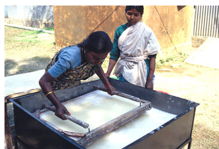
Figure 10: Forming using the dipping method with a bamboo frame. Photo: Zul / Practical Action.
