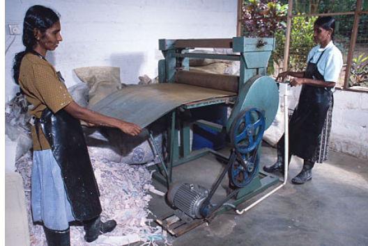
Figure 15: Jayawathi Yahampath and Shanthi Dassanayake calendering the dry paper, Sri Lanka. Photo: Zul / Practical Action.
