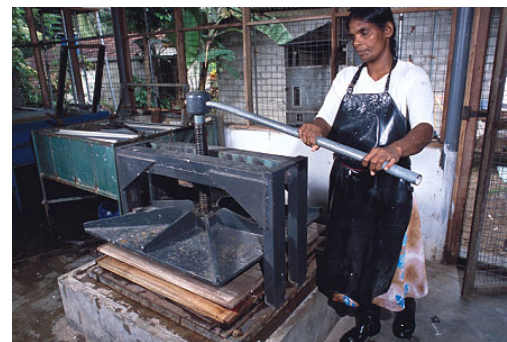
Figure 12: Honnathara. E D Karunawathi using a screw-press to remove excess water. Photo: Zul / Practical Action.
