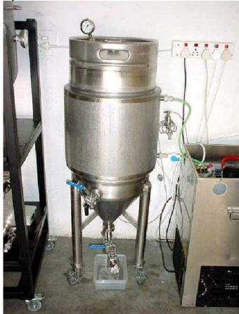
Fig 10. – Conical fermenter
