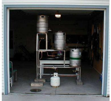
Fig 11. – Three tier gravity feed set-up
