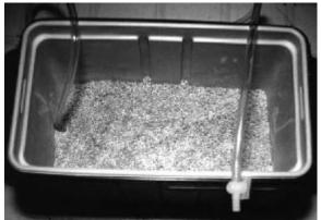
Figure 93: The lautering manifold is now installed in the bottom of the cooler. Designs will vary depending on what you have to work with.
