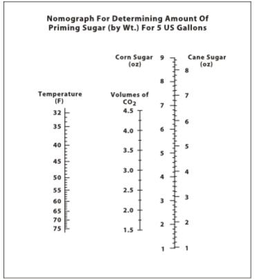
Figure 65- Nomograph for determining more precise amounts of priming sugar. To use the nomograph, draw a line from the temperature of your beer through the Volumes of CO2 that you want, to the scale for sugar. The intersection of your line and the sugar scale gives the weight of either corn or cane sugar in ounces to be added to five gallons of beer to achieve the desired carbonation level. Here is a list of typical volumes of CO2 for various beer styles:
