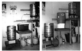
Figures 94 & 95: These two types of mash/lauter tun coolers are part of a three tier, gravity fed brewing system. A three tier set-up is not required when using a cooler, it just happens to be the way I do it. More often brewers use the cooler in
