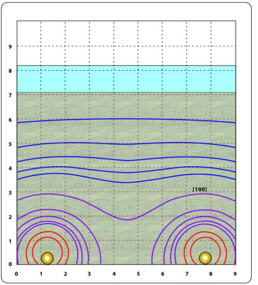
Figure 171: 2 drains spaced at 6 inches apart. Note that the flow has be vectored away from the center and is concentrated near the walls.
