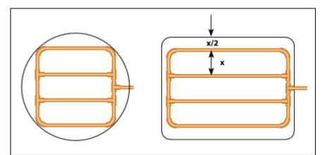
Figure 165 - Design to make the best use of the space. The manifolds should fit the bottom of the cooler, covering the most area possible and not move around. Also,
