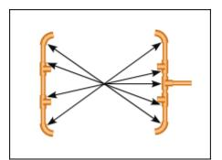
Figure 166 - A useful design for rigid tubing manifolds. Solder or crimp the indicated connections but leave the other connections for the straight tubes free. This allows easy disassembly for removal and cleaning. Be sure to completely clean the manifold of flux from soldering before use.
