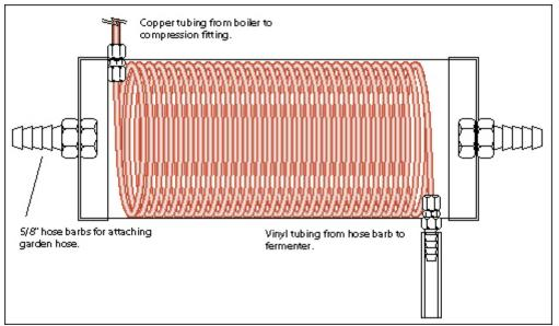
Figure 160 - Hybrid chiller inside a PVC pipe.
