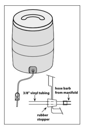
Figure 161 - Beverage Cooler and Detail of Modified Spigot Hole. A suggested method for securing the manifold outlet through the cooler spigot hole is shown here. Threaded plastic or brass bulkhead fittings can also be used.
