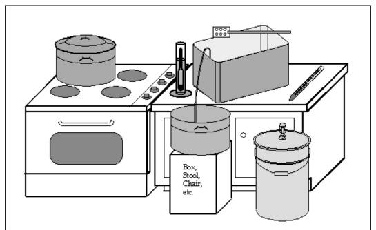
Figure 90 - Common Mashing Setup- This picture depicts what is probably the most common home mashing setup. The Mash/Lauter Tun sits on the counter near the stove and two large pots are used to prepare the sparge water and receive the wort.
