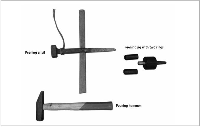
Figure 5. A peening hammer, peening jig, and a peening anvil.
