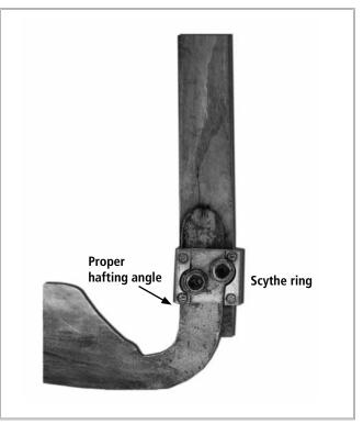
Figure 4. The proper hafting angle in which the tang hangs snug against the blade side of the scythe ring.
