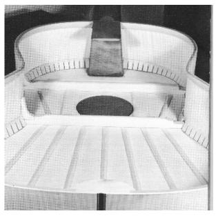
This takes place in a fixture which helps align the parts. You now have a rather rough object which is in the approximate shape of a guitar. It doesn't sound very good if you tap it now.
