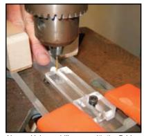
Above: Using a drill press with the Bridge Pin Groover to groove a slot into a pin.
