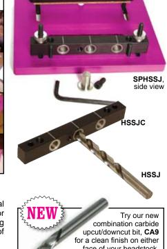
combination carbide upcut/downcut bit, **CA9** for a clean finish on either face of your headstock. It's a little more expensive, but well worth it. We use this bit regularly in our shop. It has a ¼" 2 flute upcut for ¾6" of the bit then it transitions to a 2 flute downcut for the remaining %6" of the cutting length. Overall length 2½", Total LOC: .75"
