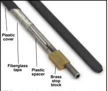
TRS rod with heat-shrink tubing cut back to expose (white) plastic spacer between rods and fiberglass tape wrap. Note the brass stop block and the specially made LMI nut.
