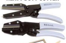
These cutting tools have a flat sturdy anvil which provides a surface for making a perfect binding or purfling cut. The stainless steel cutter is removable for easy sharpening and the offset pivot makes for smooth easy cuts. Besides making trimming your binding a breeze, these cutters are great for a multitude of tasks around the shop. The jaws on the 21/2" blades open 1" and the 3%" open 11/2".
