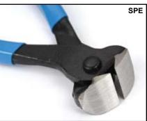
use only for cutting fretwire. These cutters work great on nickel/silver wire, but don't hold their edge long against stainless steel. We recommend our **SPSC** diagonal cutters for stainless steel wire.
