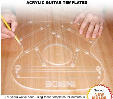
For years we've been using these templates for numerous tasks in our shop and now we are making them available to our customers. Each template is the precise outline of the guitar. Each has the top bracing and bridge placement etched on the template
