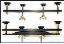
Fox bridge clamps (top-bottom): Classical clamp, steel string clamp, and steel string clamp attached to bridge.
