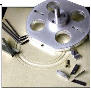
Drill Press Rosette Cutter with tool blanks, shims, drill bushing adjustment wrenches, and cutter set.
