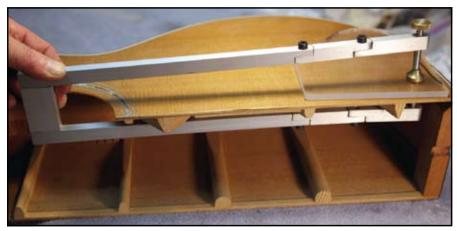
Above: X-section of the articulated clamp in use. Below: CLAC showing the articulating joints.
