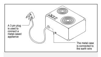
Figure 15-5 Metal-cased devices should be earthed
