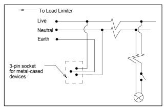
Figure 15-6 An earth connection must be provided if metal cased loads are likely to be connected.
