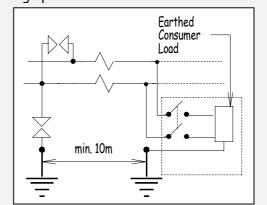
Figure 16-3 Ensure that the consumer earth electrode (if used) is at least ten metres from the neutral-earth arrestor electrode.
