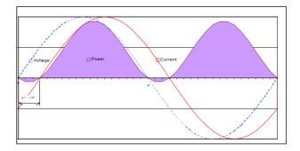
Figure 19-5 General circuits are combinations of resistance, capacitance and inductance. Here the current lags the voltage by 30° as the load is both resistive and inductive. The power factor  $(\cos\phi)$  is close to 1 and the amount of reactive power consumed is small but must still be supplied by the generator.
