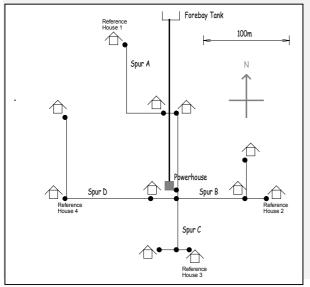
Figure 14-2 Radial spread distribution system
