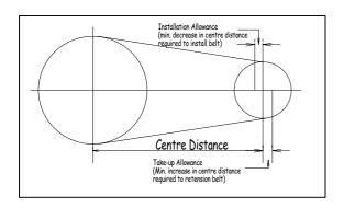
Figure 13-7 Measurement of centre distance
