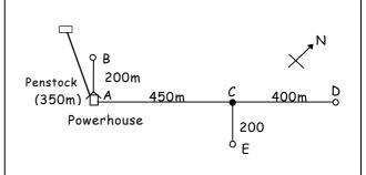
Figure 14-11 Distribution system with load "clusters" at the end of spurs
