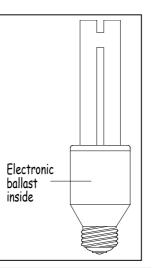
usually contained in the base of the lamp. The design allows the lamp to be fitted to a conventional socket, with either a bayonet (BS) or Edison screw (ES) fitting. You can usually tell if an inductive ballast is fitted as the lamps are heavier.
