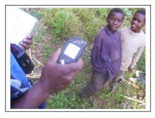
Figure 7-1 Head measurement using a digital altimeter in Kenya
