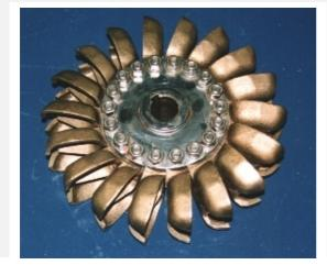
Figure 8-5 Locally Manufactured Pelton p.c.d.180 mm (Sri Lanka)
