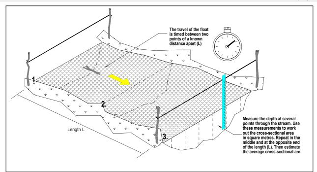
Figure 7-6 The float method of flow measurement
