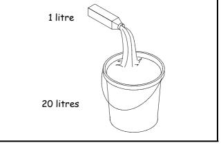
Figure 7-4 Use a small container of known volume to find the volume of a larger one.
