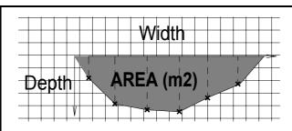
Figure 7-5 Squared paper can be used to help estimate the cross-sectional area
